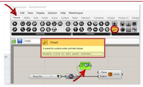
First we will display our number. We can do that with a **Panel** component. This is a very versatile component as it can be used to *input* values and display *output* data as in this case. We attach it to the **Number** output node.
