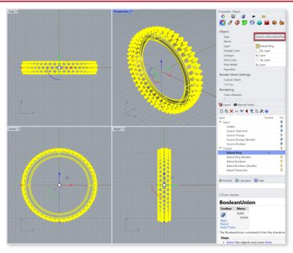
Select all the *objects* on the **Baked Ring** Layer and run the **BooleanUnion** command. After a few seconds, you should have a successful *closed solid polysurface*.
