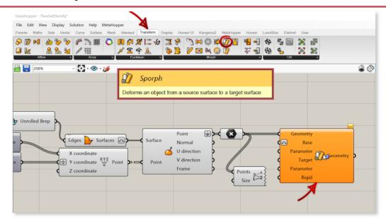
We have finally arrived to the crux of our project. The **Sporph** component allows us to bring our flattened points back into the 3-D realm. Connect our *flattened* point data into the *Geometry input*.
