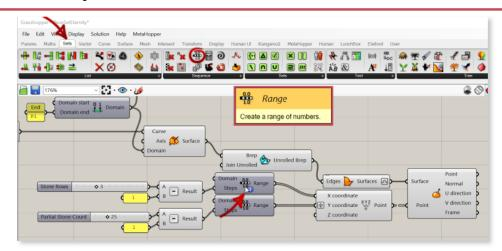
First we need a **Construct Point** component. Now say I want **three rows** with **25 diamonds** each. We can use a **Range** component to supply our points. This component allows us to set **Steps** which divides our *Domain* (0-1). Because there will be a point on either end of our *step* (*division*) we will have one additional point.
