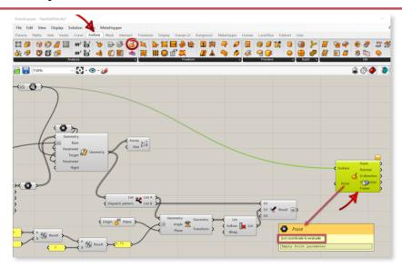
OK. We have our point locations set. The final thing we need to do for our point layout is prepare the *normal* directions for our stones or here specifically we will use the *Frame output* of another **Evaluate Surface** component.
