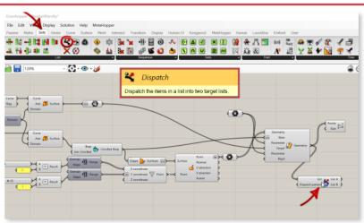
We want to shift the points in the middle row so that our diamonds are staggered from each other. Here I use the **Dispatch** component to *split* our point list based on a pattern.
