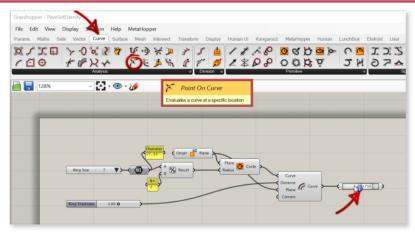
There is a wonderful component called Point On Curve. We can use this to get a point along the curve. For instance a value of .250 would place a point exactly at the quarter mark of the curve.
