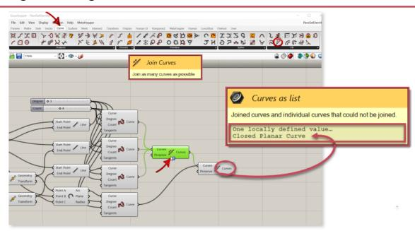
Now use the **Join Curves** component but it works best to join the lines first then run the component a second time adding the arc.
