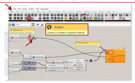
We are going to take *Unrolled Brep* output from the **Unroll Brep** component and feed that into our *Base* input (set it to *Reparametrize* the data).
