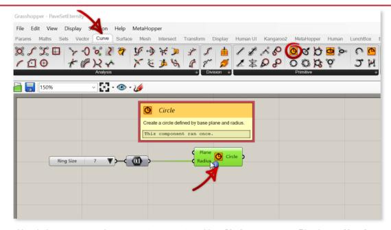
Now let's use our number to create geometry with a **Circle** component. Plug in our **Number** output into the **Radius** input.
