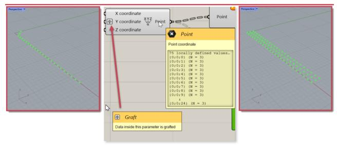
Turn on *Graft* (up arrow) for the *Y coordinate* input. The illustration above shows our points without grafting (left). This has a total of 25 points. Our goal is to have 25 groups of 3 points for a total of 75 points (right). Grafting is a way to group our data differently. Grafting either the X or the Y coordinate (not both) will group our points in a way that gives us 75 points.
