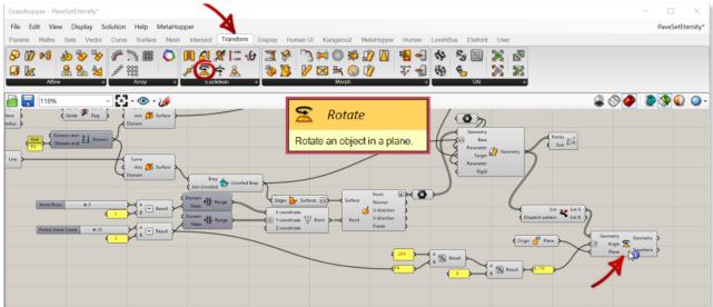
Now that we have our *List A output* we want to plug it into the **Rotate** component (*Geometry input*). Note that **GH** work natively with *radians* not *degrees*. Be sure to change the *Angle input* to accept *Degree* data.
