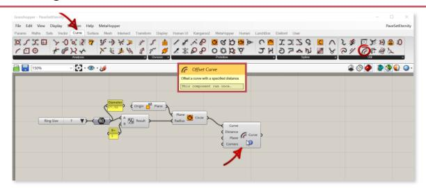
Similar to Rhino, to create the *thickness* of the ring, we use the **Offset Curve** component. We want to feed it three things.
