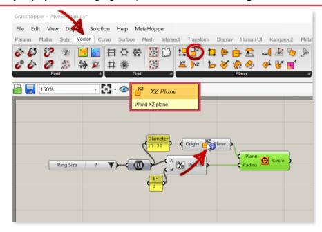
To change the plane all we need to do is drag an **XZ Plane** component and plug it into the **Plane** input of our **Circle** component and we have ourselves a functioning *finger rail*.
