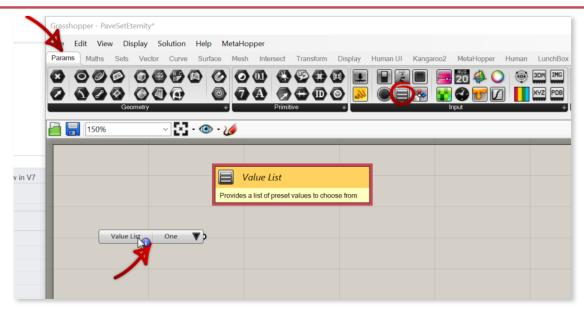
The tools for **GH** are called **Components**. They are found in the **Collection of components** (below the **Main menu bar**). <u>Click and drag</u> the required component onto the **GH canvas**. As you get to know their names you may load each component using a short cut, which is to <u>double-click</u> the canvas and type its name into the resulting <u>search box</u>.
