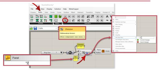
The **Division** component is needed to divide our number in half (converting *diameter* to *radius*). We want our *diameter* as the *Dividend (A)* and our *Divisor (B)* is 2.
