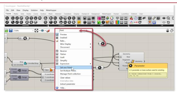
The **Parameter** Inputs need to correspond. This represents UV space (similar to picking near a corner for Flow Along Surface). Here I want to set both to (0,0,0).
