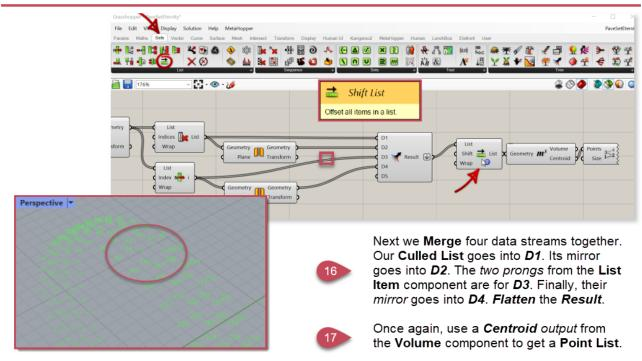
You may notice that the preview has 0 and 1 out of sequence on the list. This is easily fixed with **Shift** List component. Enter a value of **2** for the *Shift* input.
