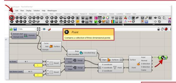
We need to hook up a **Point** component to the **Point** output of our **Evaluate Surface** component. This is a container that will store the data of our 75 points.
