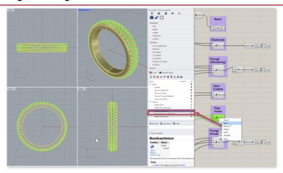
Again for a production model ring Bake the Pilot Holes by right-clicking and selecting Bake.
