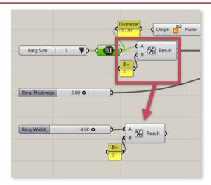
Creating a profile in Rhino, may start by using a **Single Line** cmd (from **Y=0**) using **BothSides** in the **command line**, then entering a **half value** of the line's length. The concept is similar in **GH**. As we have a number representing the width of our profile we can simply divide that number for our **positive** Y coordinate and find its **negative** result for the **negative** Y coordinate.
