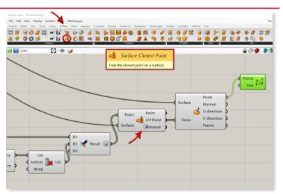
...we insert a Surface Closest Point component to get our *UV coordinates*. The *Surface input* is yet again the one from (step 3; pg 21). Plug our merged point Result into the **Point** input.
