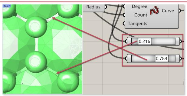
Revisit our last two **Point On Curve** components (previously set at .210 and .790). We can adjust the *gap* between the *middle row* and *outside rows*.
