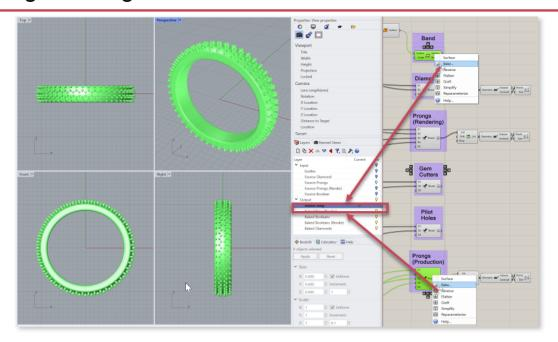
We have to **Bake** our GH results to create the geometry for Rhino. For a *production* model ring **Bake** the **Band** and the **Prongs (Production)** by <u>right-clicking</u> each component separately.
