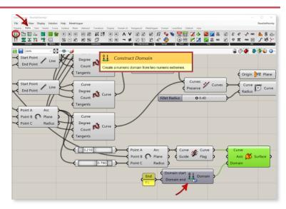
We assign this by plugging a Construct Domain component into the *Domain input*. The *Domain start* remains 0. For the *Domain end* we want to use  $\pi$  (Pi) not 2  $\pi$  (the full circumference).
