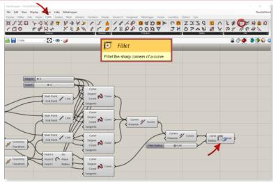
Now we can fillet the curve to our liking. Drag in the **Fillet** component. The *radius* can be changed later so we want to input a **Number Slider** (with 2 *decimal places*) for the **Radius** input.
