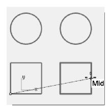
**5** For the **Next point**, move your cursor close to the midpoint of the vertical line at the right side of the square on the right, pick when the marker snaps to the midpoint.
