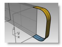
**5** For the **Extrusion distance**, type **.375** and press **Enter**.
