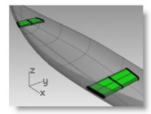
A surface is fitted over the curves that fit exactly with the shape of the hull.
