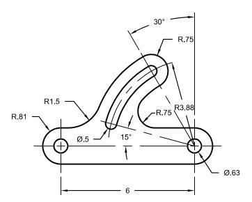
**3** Use Extrude Planar Curve > Straight on the Solid menu to create the 3-D part. The extrusion thickness is 0.5.
