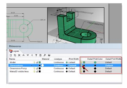
All the objects on the layer that was turned off in the Detail On column are not visible in the Perspective view but remain visible in all other details.
