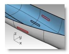
Project uses the current construction plane to determine the direction of projection. Make sure you select the curves and surface to project onto in the Front viewport.
