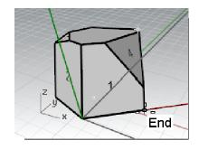
**4** For the **Cplane orientation**, snap to the upper left corner of the surface labeled as 1.
