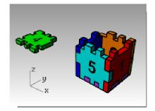
4 Now use Gumball to move the final **Piece 4** into position on the top of the box using the **Axis plane** indicator.
