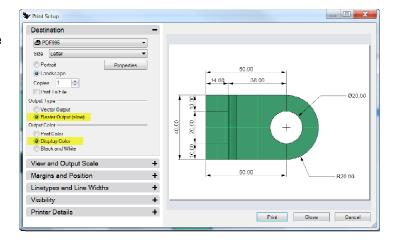
4 In the View and Output Scale area, select Scale of 2:1, On Paper 1.0 Millimeter, and In Model 0.5 Millimeter.
