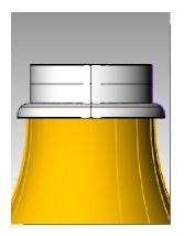
6 Use the **BooleanUnion** command (Solid menu > Union) to join the two polysurfaces together.
