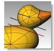
For the **Object to** trim, pick the bottom of the head and the top of the body.
