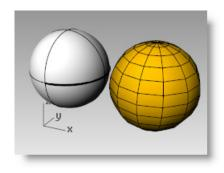
A Sphere surface and mesh sphere object.
