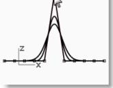
Individual points have more influence on a small area of the curve with degree 3 curves, while points have greater influence over a wider span of the curve with degree 5 curves.
