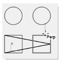
The marker snaps to a point making a perpendicular to the previous point.
