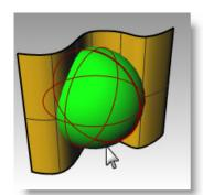
The sphere is separated into two pieces precisely where the surface intersects it.
