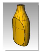
**Note:** It is possible to create a hollowed out shell from a solid polysurface, like this bottle. The command for doing this is **Shell**.
