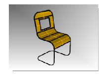
**9** Highlight the seat surfaces. Using the Layer pane in the Status bar, select the Seat layer.
