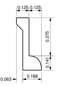
**6** Use the **Move** command (*Transform menu > Move*) to move the profile from the midpoint of the bottom edge to the midpoint of the top of the bottle.
