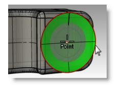
9 Use the BooleanDifference command (Solid menu > Difference) to remove the surface from the top of the phone.
