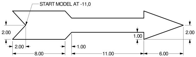
Draw the arrow with a polyline, using a combination of absolute coordinates (x,y), relative coordinates (Rx,y), polar coordinates (Rdistance < angle), and distance constraint.
