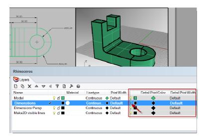
3 Double-click the Perspective detail to deactivate. Highlight the boundary edge of the detail. In Object Properties set the Print Width to No Print
