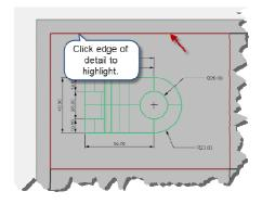
3 In the **Scale** area, set **1.0 mm** on layout equal to **1 mm** in model.
