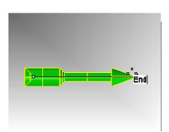
For the Point to bend through, drag the cursor down and pick a point.
