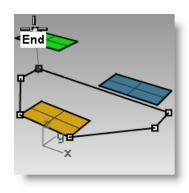
The Project constraint forces all the segments of the polyline onto the construction plane. The resulting polyline is planar.
