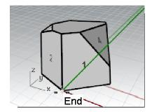
**3** For the **X axis direction**, snap to the lower right corner of the surface labeled as 1.
