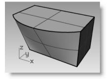
**Hint:** Use the **What** command to confirm that offset polysurface is valid, closed solid.
