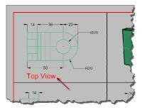
5 In the **Text** dialog set the **Height** to **7mm** and type **Top View**.
