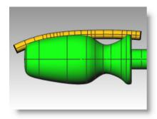
**10** Use the **ArrayPolar** command to make copies of the pipe around the handle.
