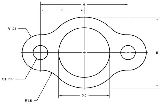
3 Use **Extrude Planar Curve > Straight** on the **Solid** menu to create the 3-D part. The extrusion thickness is **.125**.
