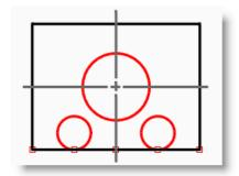
A circle is created with the two points you picked as the diameter, and the diameter was constrained to a value of 4.
