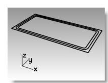
To change the type of corner, click Corner on the command line to toggle from circular rounded corners to conic rounded corners.
