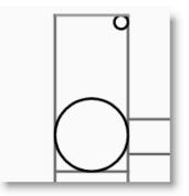
**5** Use the **Arc** command (*Curve menu > Arc > Tangent, Tangent, Radius*) to create arcs that are tangent to the two circles.
