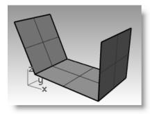
4 For the **Height**, use **SmartTrack** to track a point from the top of the vertical plane. Drag the tracking point until the surface is tilted slightly and click.
